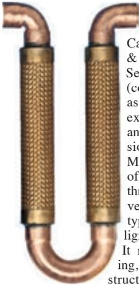
This means that the Metraloop complies with California's Health & Safety Code Section 116875 (commonly known as AB 1953). An extremely flexible and compact expansion joint, the Metraloop has none of the pressure thrust loads of conventional bellows-type joints and negligible spring rates.
