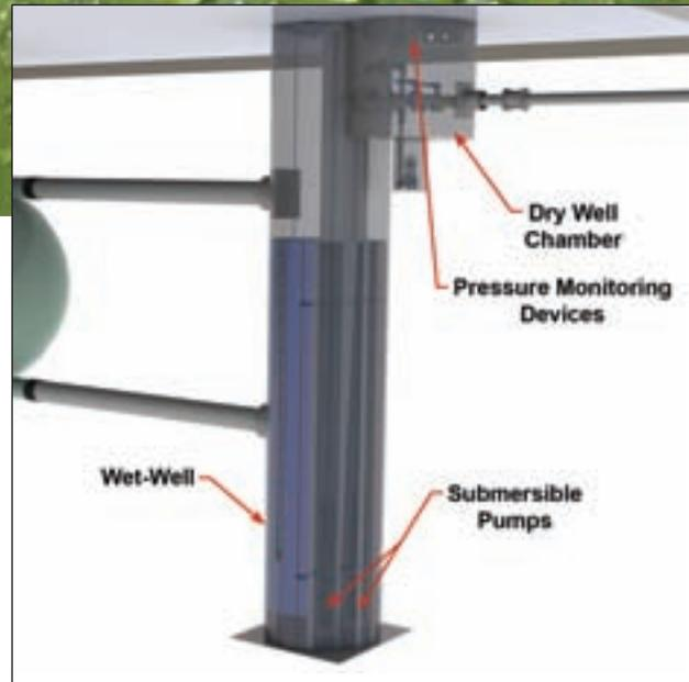
*The pressurization station includes two variable speed submersible pumps, each designed to pressurize the rainwater at a peak flow-rate of 80 gpm, with a target output-pressure of 80 psi and a combined peak flow of 160 gpm.*
